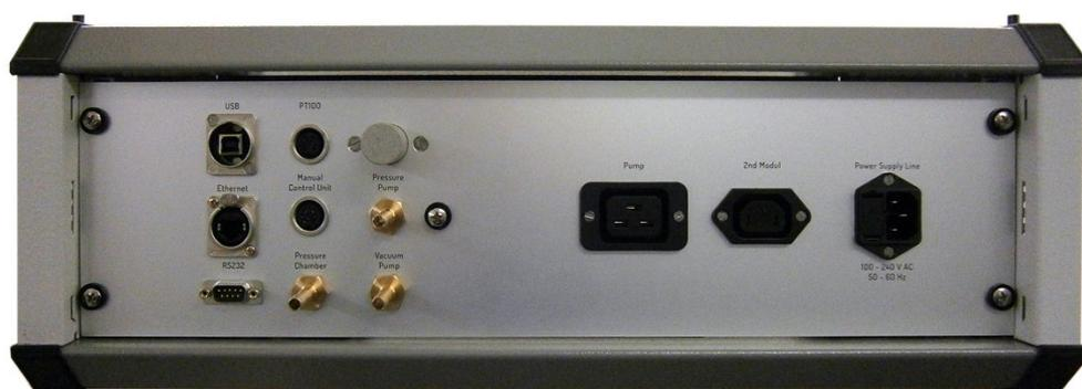
For automatic operation a PC or Laptop will be used. The relevant plug for the connection of the PC is placed at the back plate.
